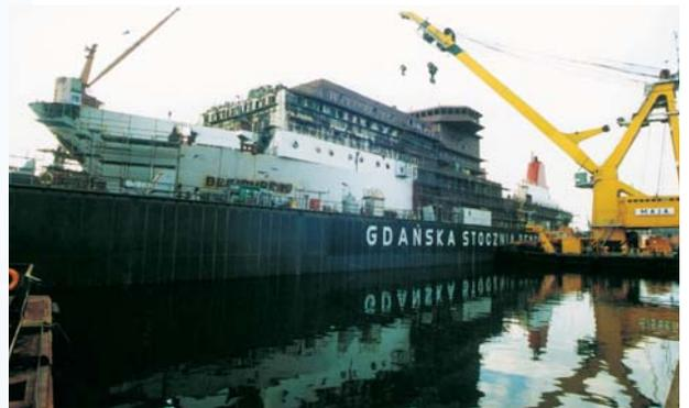
As a result of the conversion, the breadth of each ship was increased from 20.5 to 23.3 m and the draft from 6.45 to 7.23 m whilst the load capacity was reduced from 6.704 to 4.500 dwt.
